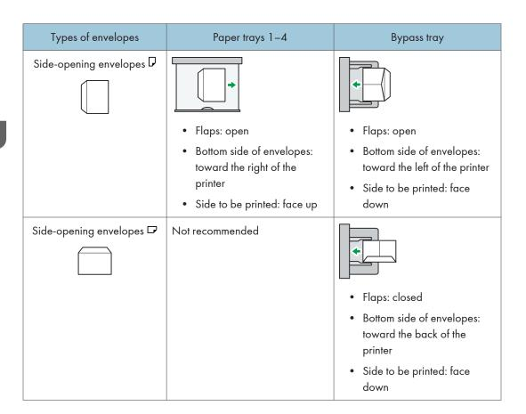
When loading envelopes, use both User Tools and the printer driver to select "Envelope" as the paper type and specify the thickness of the envelopes. For details, see p.61 "Printing on Envelopes", Printer.
